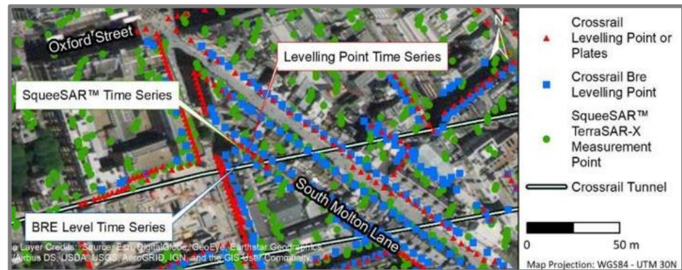
Verification of in-situ instrumentation (levelling in this case)
