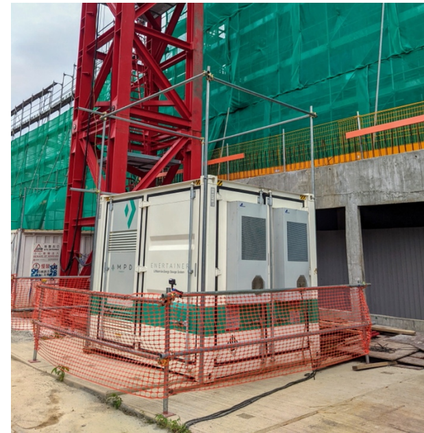
Enertainer powering a tower crane lifting a heavy MiC module
